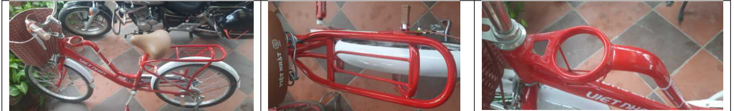
Viet Nhat bike with welded steel front and rear seats
